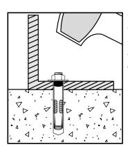
Drive the anchor through the fixture into the anchor hole until the head is firmly seated against the fixture. Be sure the anchor is driven to the required embedment depth.
