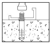
Insert the anchor through the fixture into the hole. Set the anchor by driving the anchor body over the plug. Be sure the anchor is driven to the required embedment depth. A nut and washer (to be supplied separately) is applied to secure the fixture.
