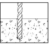
Drill a hole into the base material to a depth that equals the embedment required. The tolerances of the drill bit used should meet the requirements of ANSI Standard B212.15. Do not over drill the hole. Blow the hole clean of dust and other material.
