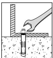
Tighten the anchor by turning the nut or head 3 to 5 turns past finger tight or by applying the guide installation torque from the finger tight position.
