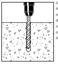
Using the proper diameter bit, drill a hole into the base material to a depth of at least 1/2" or one anchor diameter deeper than the embedment required. The tolerances of the drill bit used should meet the requirements of ANSI Standard B212.15.
