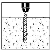
Using the proper diameter bit, drill a hole into the base material to a depth of at least 1/2" or one anchor diameter deeper than the embedment required. The tolerances of the drill bit used should meet the requirements of ANSI Standard B212.15.
