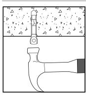
Using the proper diameter bit, drive the anchor into the hole until the head is firmly seated against the base material. Be sure the anchor is driven to the required embedment depth.
