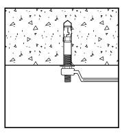
Run the nut and washer up to the concrete surface and tighten the anchor by turning the nut 3 to 5 turns past finger tight or by applying the guide installation torque from the finger tight position.
