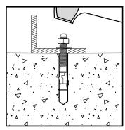
Position the washer on the anchor and thread on the nut. Drive the anchor through the fixture into the anchor hole until the nut and washer are firmly seated against the fixture. Be sure the anchor is driven to the required embedment depth.
