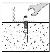
Tighten the anchor by turning the nut 3 to 5 turns past finger tight or by applying the guide installation torque from the finger tight position.
