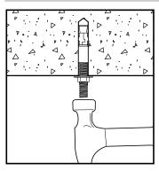
Thread the anchor onto the rod to be used along with a nut and washer. Drive the anchor into the hole until the anchor is at the required embedment depth. The anchor body should be recessed in the hole.
