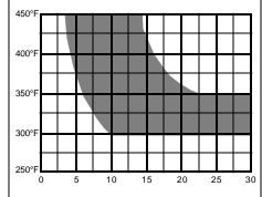
Part Time at Peak Metal Temperature (.0345 inch C.R.S. panel)
